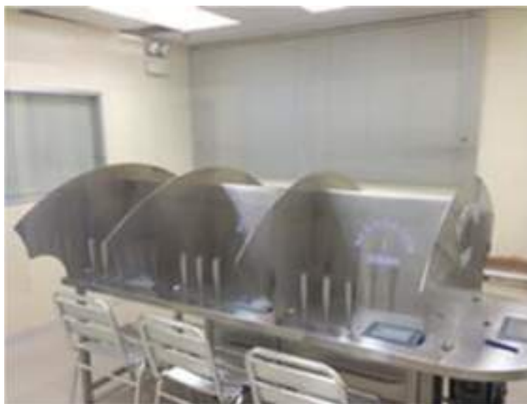
Figure 3: Olfactory Laboratory with Scentroid™ SS600 Olfactometer
